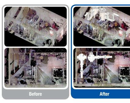
Using the scanned data obtained through the Laser 3D scanner, 3D simulation of the mounted GloEn-Patrol™ BWTS is provided to ship owners.
