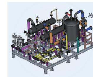
Vaporizer & Buffer Tank Module
