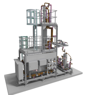
NH 3 Catch Skid
